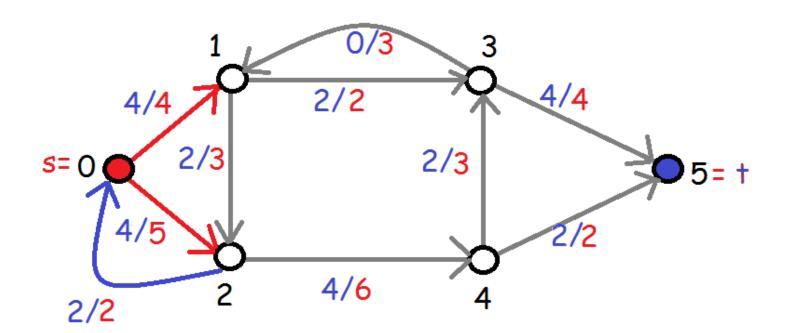
Because of conservation of flow, the amount of flow from s to t is also equal to the net amount of flow entering t.
