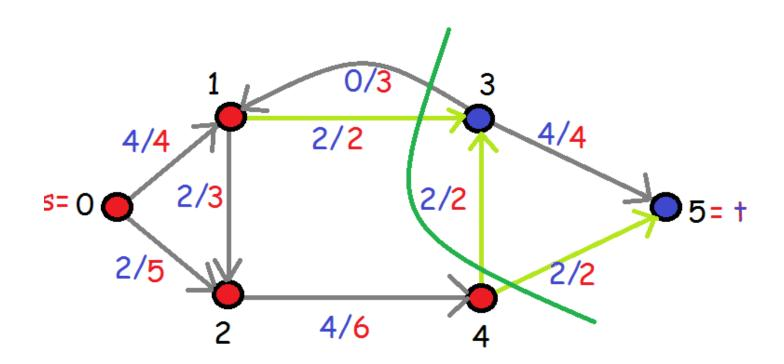
The maximum flow from s to t cannot be more than the capacity of any of the s,t-cuts. Theorem: the maximum flow equals the minimum capacity of an s,t-cut.
