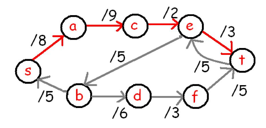
Identify augmenting path: s, a, c, e, t Capacity of path is 2.
