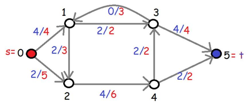
The amount of flow from s to t is equal to the net amount of flow exiting s = sum over arcs e that exit s of f(e) - sum over arcs e that enter s of f(e).
