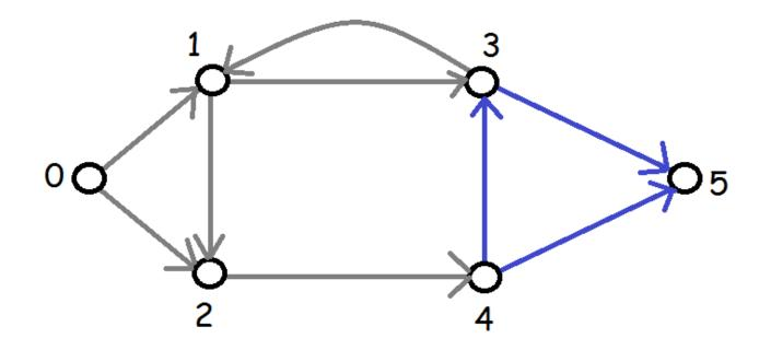
A cycle of length 3 which is not a directed cycle (arcs can be traversed in either direction):
