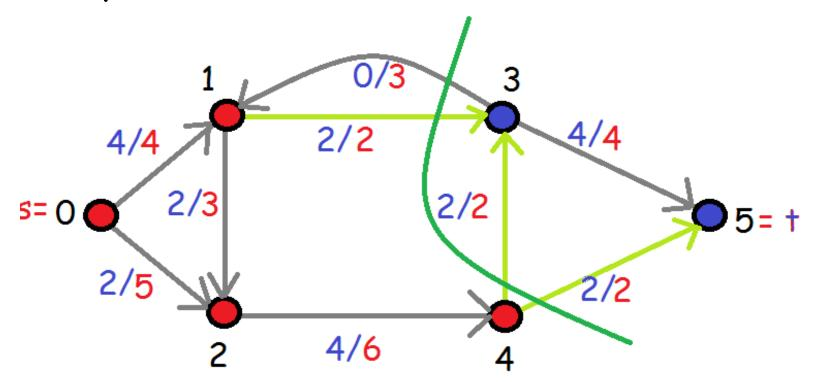
The capacity of a cut (S,T) is the sum of the capacities of the arcs in the cut.  $(S,T)=\{(1,3), (4,3), (4,5)\}$
