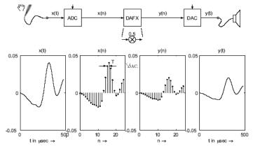
Figure 2: Signal Flow Diagram
