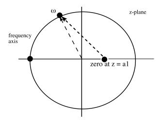
Figure 3: Evaluating the magnitude response of a simple feedforward filter. The factor  $|z - a_1|$  is the length of the vector from the zero at  $a_1$  to the point on the unit circle corresponding to the frequency  $\omega$ .
