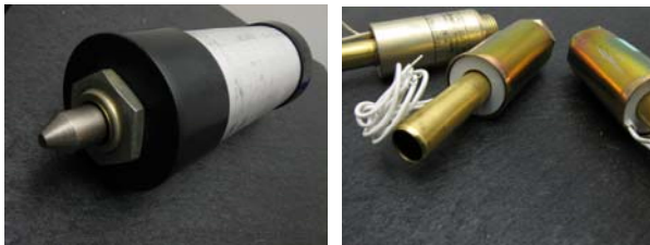
Figure 5 - Trimpin BellHop outside shell tubing (left) and inside extended tubing (right).
