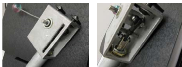
Figure 3 - Singer Hammer with added ball-joint striking mechanism.
